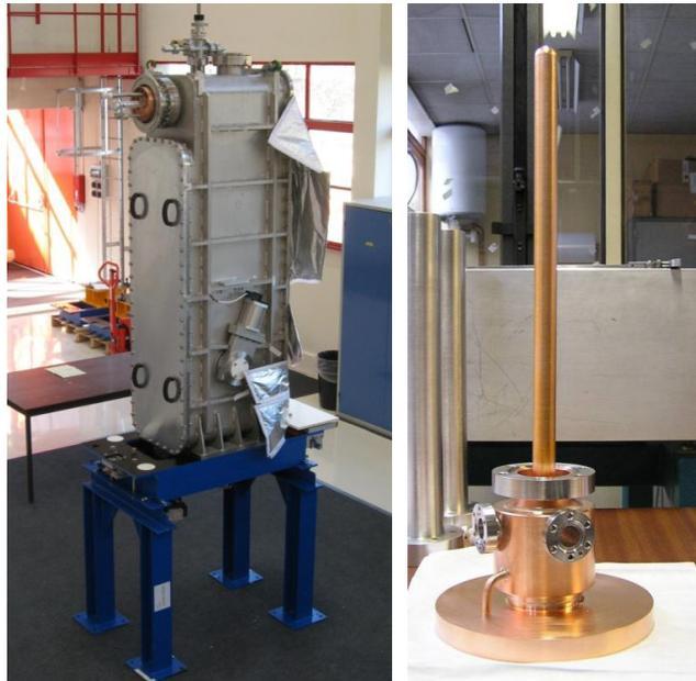
**Figure III.1.10.1 Photograph of the SPIRAL2 low-beta cryomodule that contains one cavity (the left plot) and the coupler (the right plot). This type of cryomodule and power coupler can be adopted for the RISP SCL1. (Courtesy of the SPIRAL2)**
